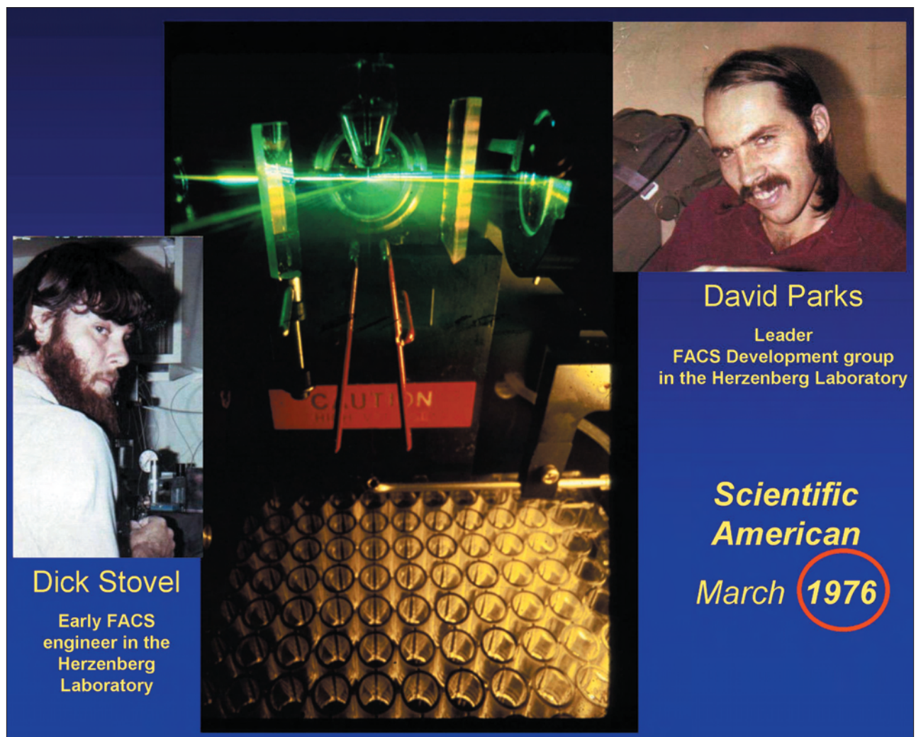
Fig. 9: FACS set-up for single-cell sorting (e.g., for cloning). Shown are a laser intersecting stream, deflection plates and a 96-well tray for collecting single droplets.
